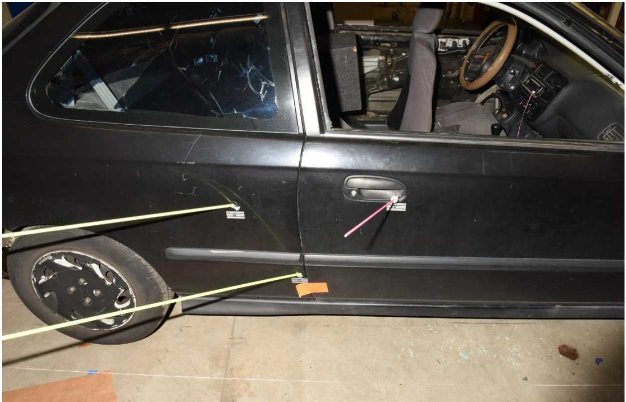
Trajectory rods, showing general direction of travel of fired bullets, inserted into the black Honda Civic Hatchback.
